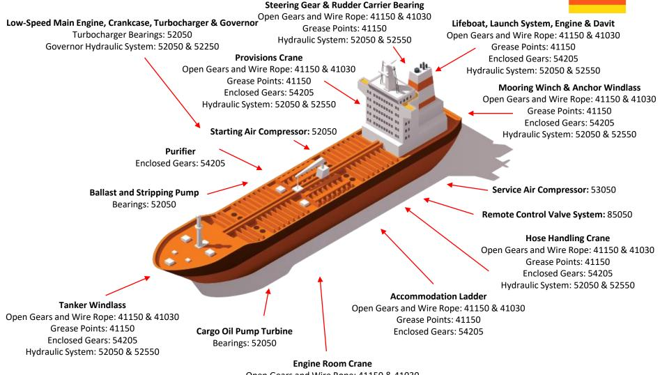
Open Gears and Wire Rope: 41150 & 41030 Grease Points: 41150 Enclosed Gears: 54105 or 54205
